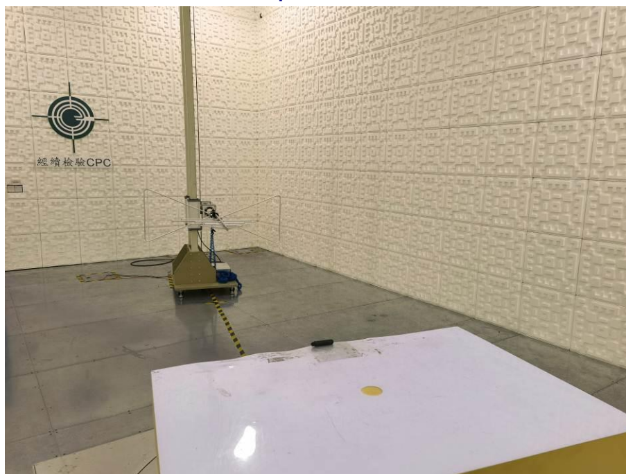
Photo of test setup for radiated disturbances
